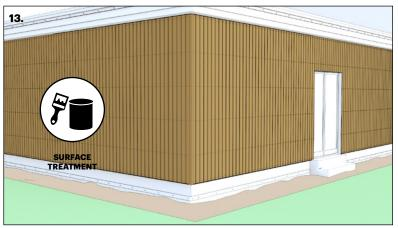
Most of the opaque paints and exterior cladding stains (with pigment included is suggested to keep the colour and protect from UV effects of the sun) are suitable for Lunawood. Please consult your local paint manufacturer. Surface treatment enables longer lifetime of the product
