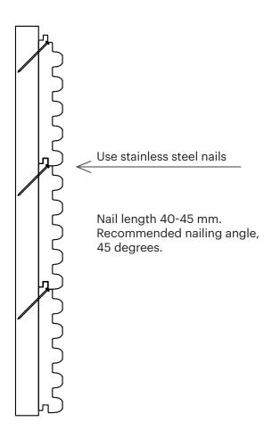
Provide adequate support structure in accordance with your local building regulations. Do not install lamps or other heavy objects directly to the product.
