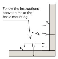
Provide adequate support structure in accordance with your local building regulations. Do not install lamps or other heavy objects directly to the product.
