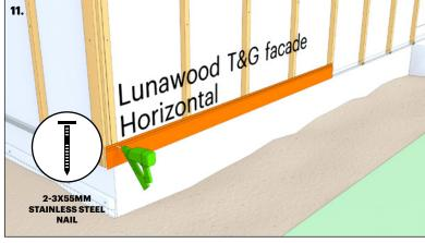
Ensure the board is well set and attach from the nailing groove.
