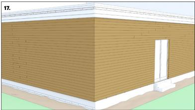
Remember to check annually the condition of the facade. The maintenance painting interval is only a rough estimate affected by structural solutions, the geographic location, and direction in which the surface faces.
