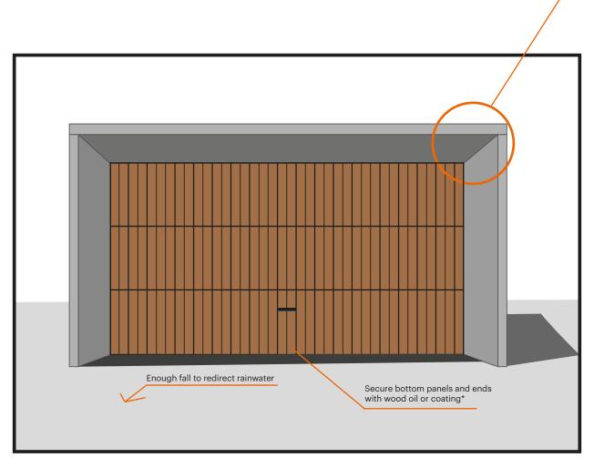
\* When Lunawood Thermowood<sup>®</sup> is treated with clear woodoil, it will turn into silver gray due to the UV light of the sun if the wood oil doesn't contain UV-protection.
