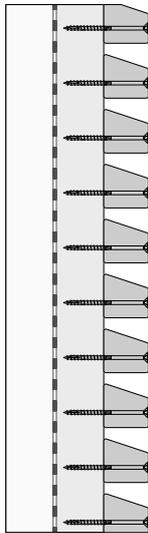
In horizontal battens cladding, profiles with a sloping top edge to allow water drainage and prevent dirt accumulation are recommended.
