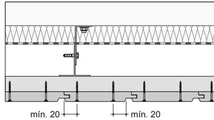
Profiles < 140 mm width can be fixed with a single screw.
