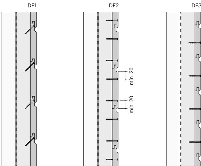
Profiles < 140 mm width can be fixed with a single screw.
