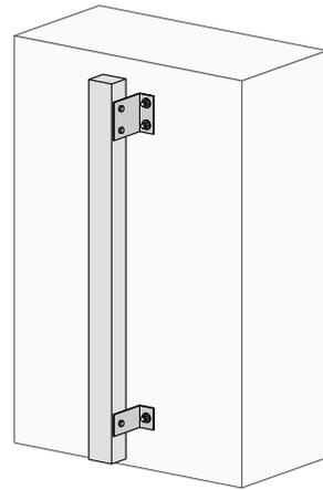
Fixing through a system of metal fastening brackets that allow adjusting the position of the battens regardless of the support wall flatness.
