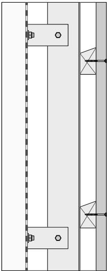
It is recommended to install the horizontal wooden support battens with a sloping top edge of at least 15° towards the interior of the cavity to shed water. [See DF1].
