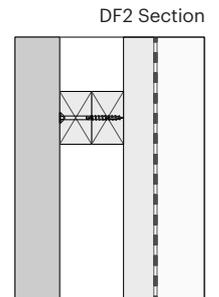
The gap between cladding battens must be equal or greater than 10 mm wide to allow fixing pre-assembled facade modules to vertical support battens.
