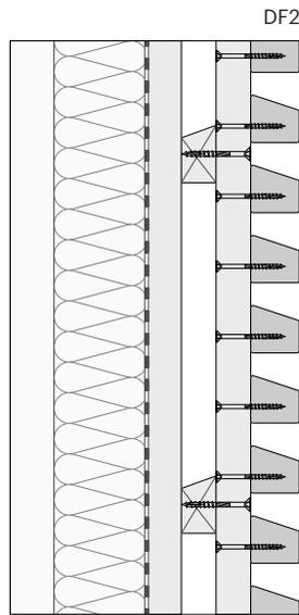
The gap between cladding battens must be equal to or greater than 20 mm wide to allow fixing pre-assembled facade modules to the structure.
