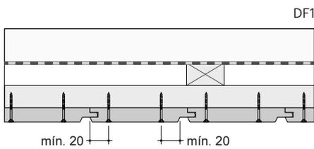
Profiles < 140 mm width can be fixed with a single screw.
