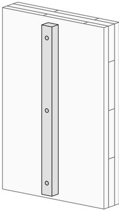
Direct fixing to a timber support wall using self-drilling screws suitable for timber made of AISI 304 (A2) stainless steel.
