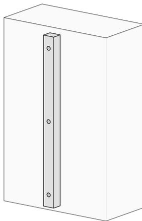
Direct fixing to a timber support wall using plastic anchors and screws suitable for use in concrete and masonry walls.
