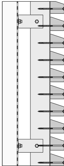
In horizontal battens cladding, profiles with a sloping top edge to allow water drainage and prevent dirt accumulation are recommended.
