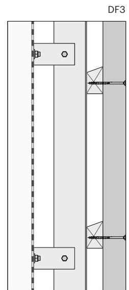
In open joints installation, the gap between battens must be equal or greater than 8 mm wide to avoid moisture traps. [See DF1].
