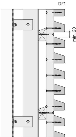
The gap between cladding battens must be equal to or greater than 20 mm wide to allow fixing pre-assembled facade modules to the structure.
