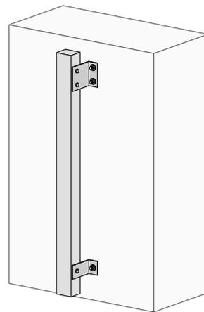
Fixing through a system of metal fastening brackets that allow adjusting the position of the battens regardless of the support wall flatness.
