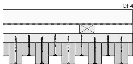
In open joints installation, the gap between battens must be equal or greater than 8 mm wide to avoid moisture traps.
