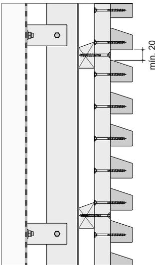
The gap between cladding battens must be equal to or greater than 20 mm wide to allow fixing pre-assembled facade modules to the structure.
