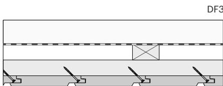
Hidden fixing only possible with HN profiles (Hidden Nailing). Use the V-shaped groove to position the screw.
