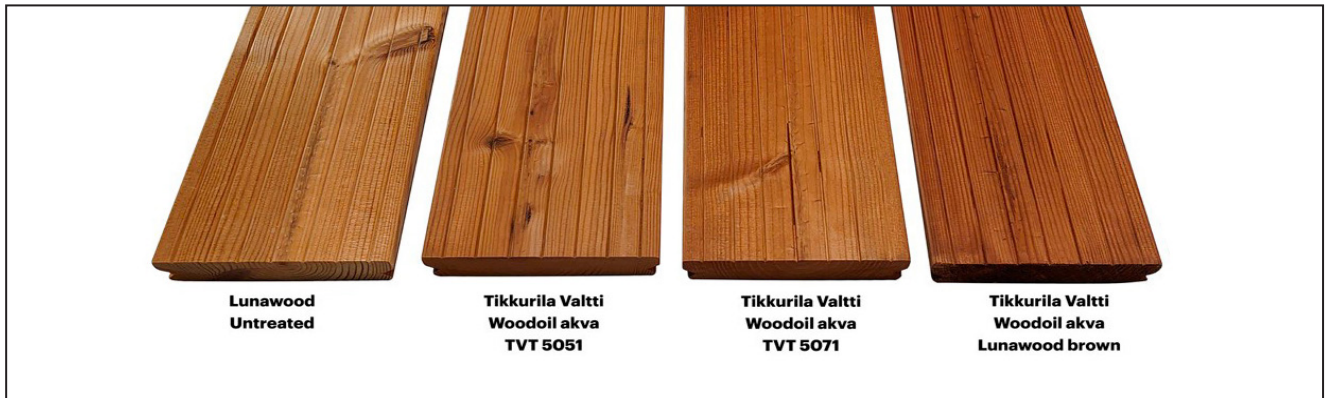
Comparison of Tikkurila oils applied to Lunawood Thermowood
