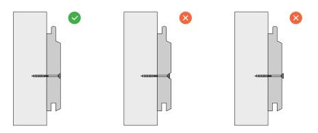
• Use one fixing at each cladding/batten intersection when the cladding profile is less than 5-1/2" wide. Use two fixings when the cladding profile is wider than 5-1/2". Always respect the edge distances recommendations.
