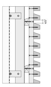
The gap between cladding battens must be equal to or greater than 4/5" wide to allow fixing pre-assembled facade modules to the structure.
