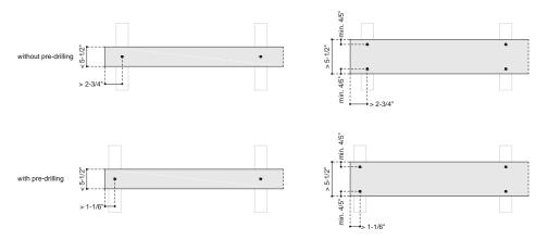
• It is recommended to fix the cladding profiles in at least 3 support battens.
