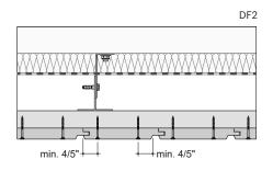
Profiles less than 5-1/2" width can be fixed with a single screw.
