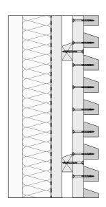
The gap between cladding battens must be equal to or greater than 4/5" wide to allow fixing pre-assembled facade modules to the structure.
