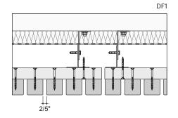
The gap between cladding battens must be equal or greater than 2/5" wide to allow fixing pre-assembled facade modules to vertical support battens.
