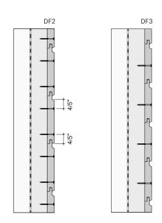
Profiles less than 5-1/2" width can be fixed with a single screw.
