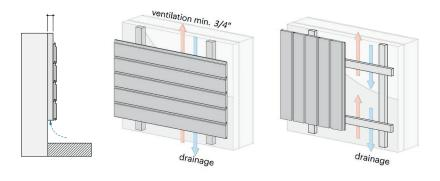
Provide an adequate ventilation cavity behind the cladding with a rainscreen. The rainscreen must provide a ¾ inch minimum air gap behind the cladding to avoid moisture traps. Do not install heavy objects directly to the product.
