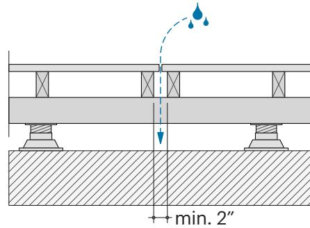
Place a spacing band that covers the entire top of the joists to stop the rise of moisture.
