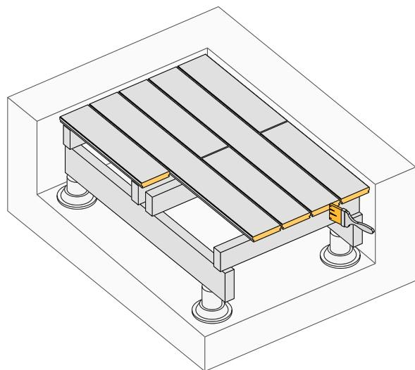
We recommend a regular surface treatment, i.e. oiling for Thermowood decking when used in applications subject to varying weather conditions. Surface treatment, will help to retain the original colour and reduce cracking and splintering that are typical to wood materials over time. More information in maintenance guide.
