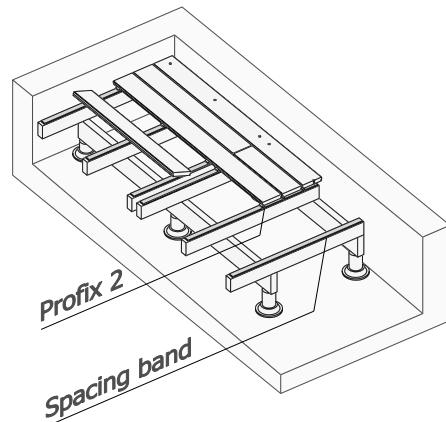
Joist-spacing depends on the thickness of the decking board
