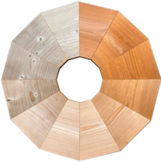
Natural greying of untreated Lunawood decking from brown to grey in 12 months (Finland).
